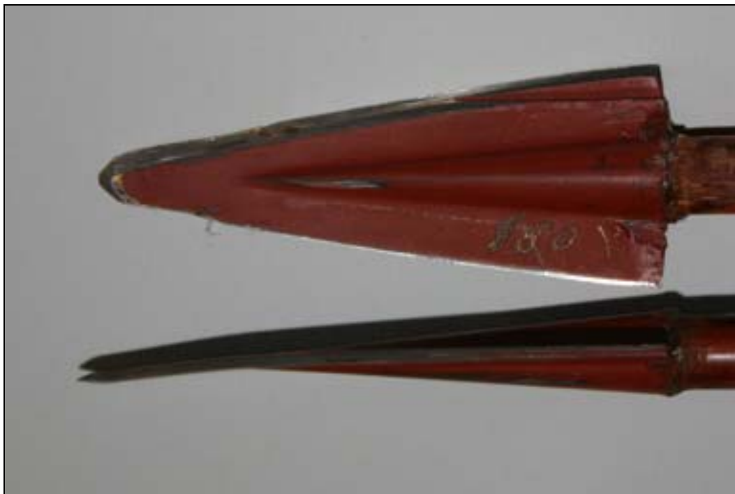
The two bent 160 grain Grizzly broadheads
