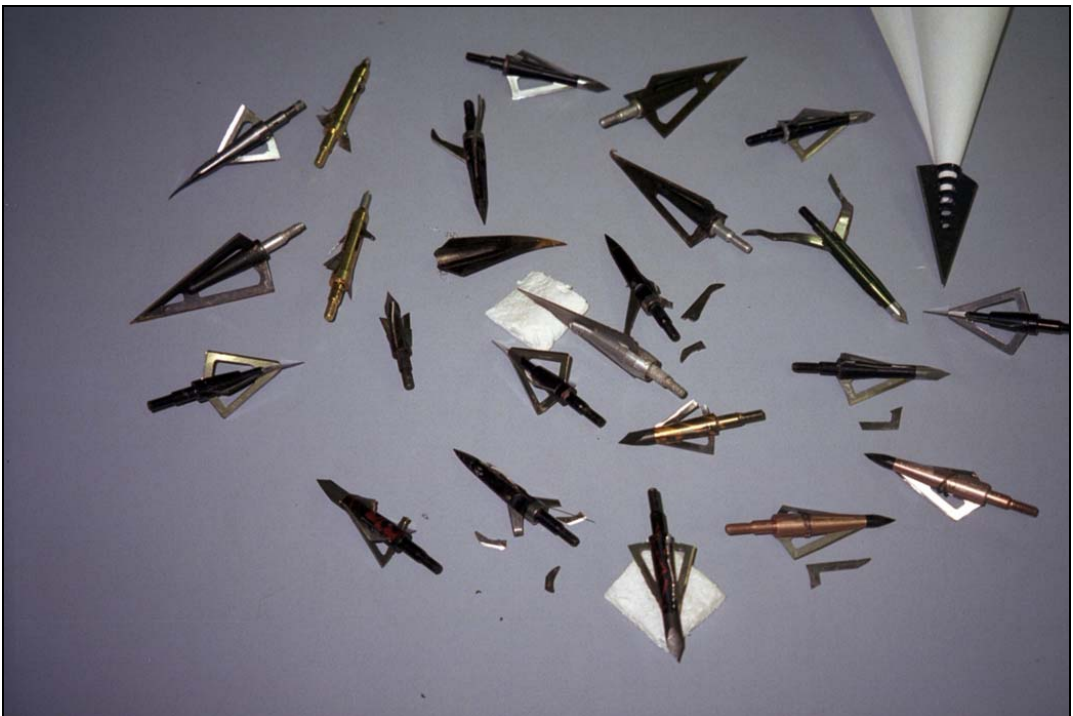
Some of the broadheads damaged during 2004 testing.
